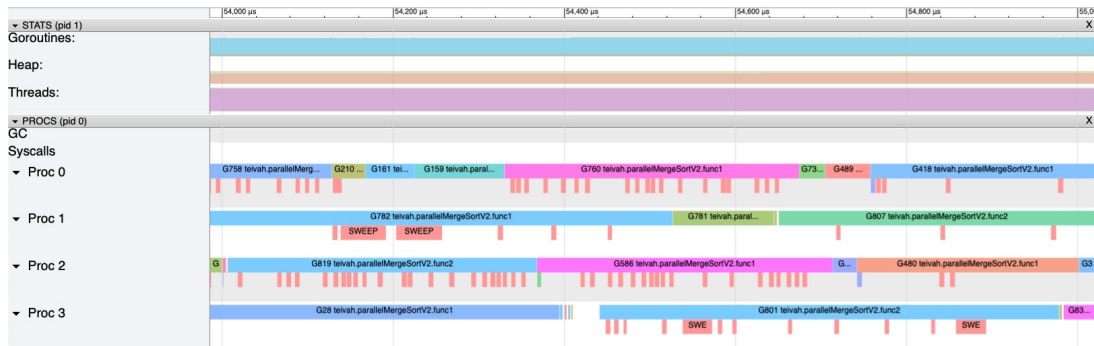
Figure 12.42 The number of white spaces has been significantly reduced, proving that the CPU is more fully occupied.
